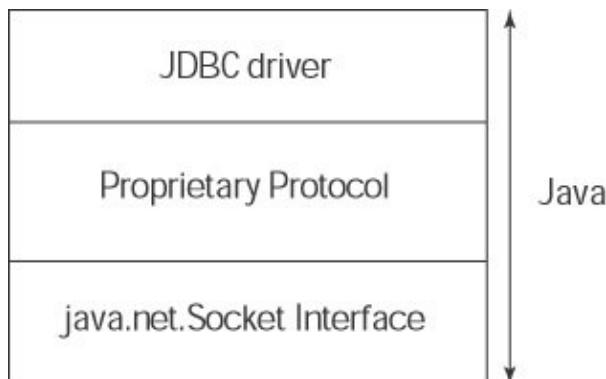
Figure 7-4: Type 4 drivers provide an interface between JDBC and the vendor's pure Java, but proprietary, API.
