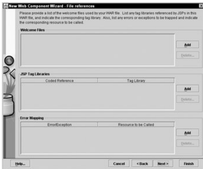
Figure A–34: Configure all of the startup and HTML files used by JSPs and servlets in this dialog.
